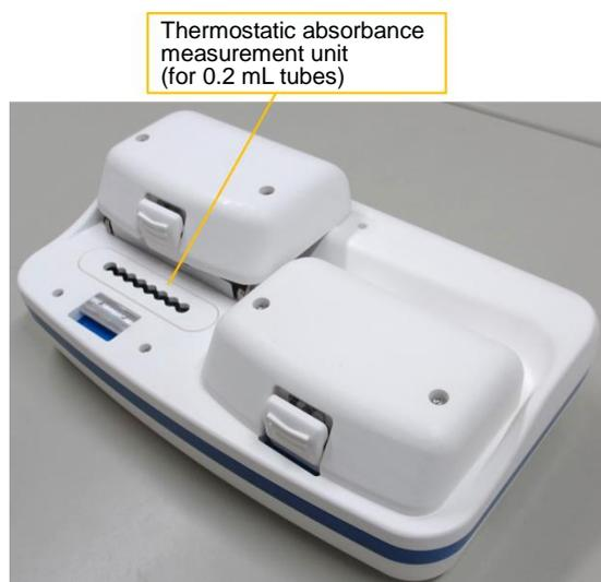
Figure 4-10: Thermostatic absorbance measurement unit (Left)
