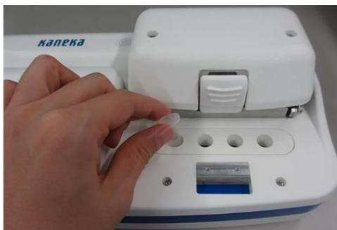
Figure 3-2: Setting a tube to the high-temperature treatment unit of the main unit
