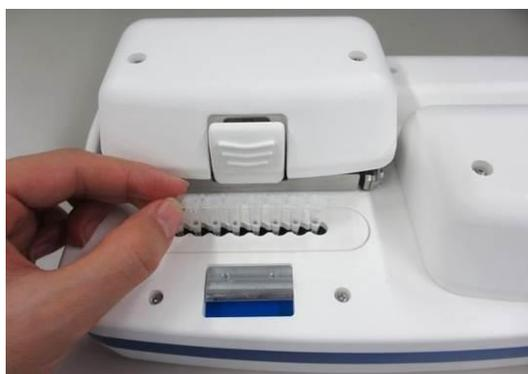
Figure 4-11: Setting a 0.2 mL tube to the thermostatic absorbance measurement unit
