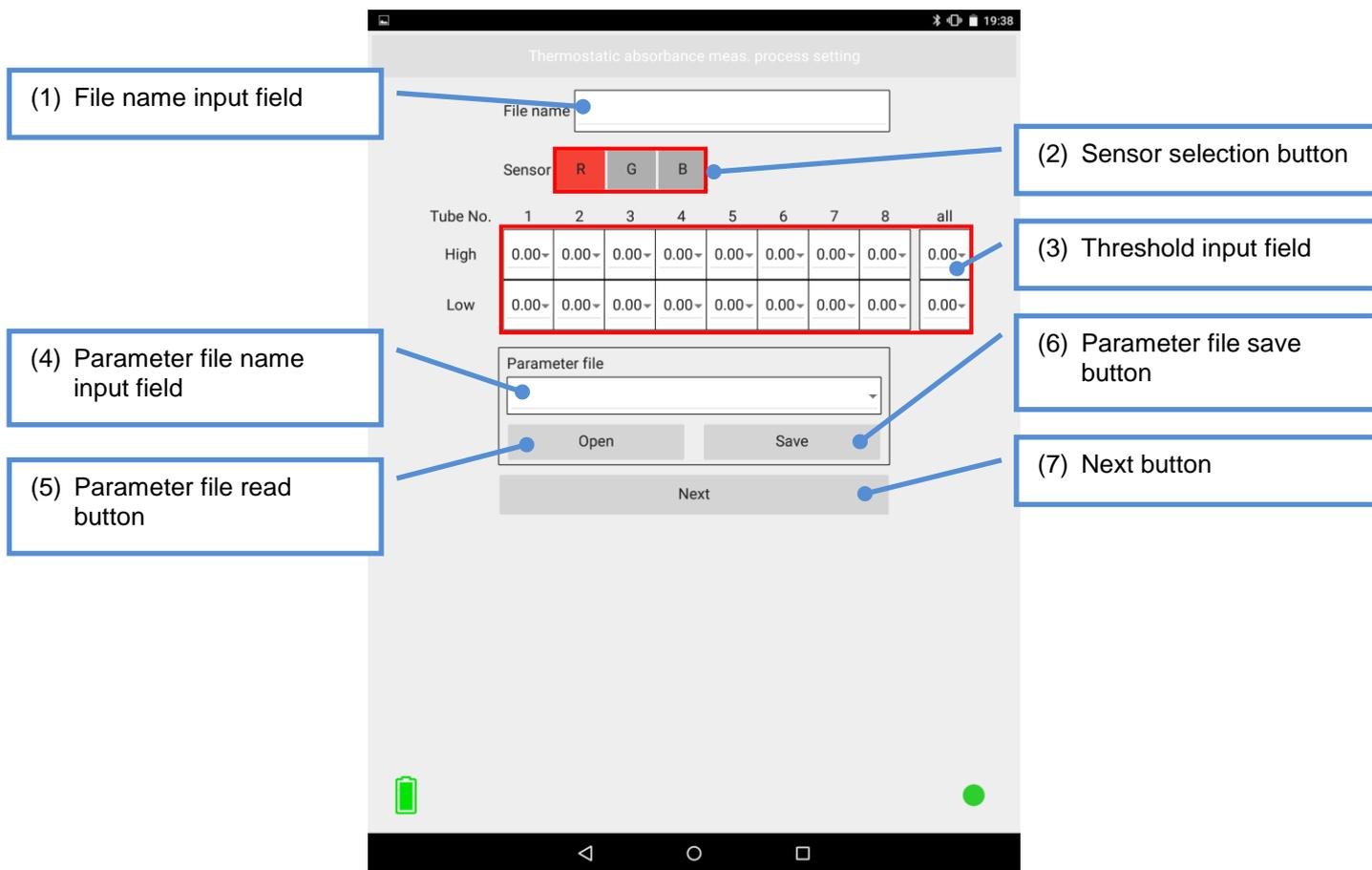
Figure 4-2: Thermostatic absorbance measurement process setting screen
