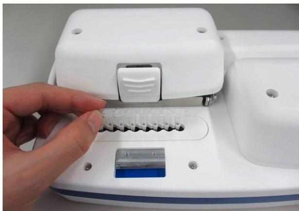
Figure 4-34: Taking tubes out of the thermostatic absorbance measurement unit
